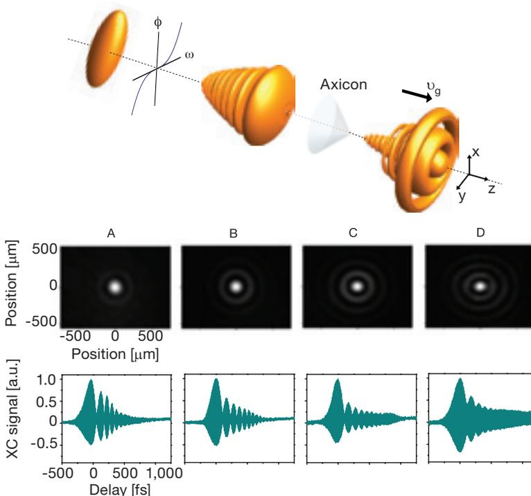
(Top) Schematic to generate Airy-Bessel wave packets. (Bottom) Propagation of an Airy-Bessel wave packet **A** initial spatial and temporal profile, **B** profiles after propagation through  $3.3 L_R$  and  $1.8 L_d$ , **C**  $5.4 L_R$  and  $3.6 L_d$ , **D**  $7.5 L_R$  and  $5.4 L_d$ . ( $L_R$  = diffraction length of a beam with a diameter of  $180\mu\text{m}$ ,  $L_d$  = dispersion length of a 100 fs pulse).
