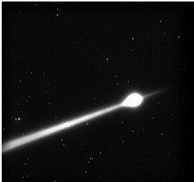
Fig. 2. Vertical propagation in the sky of the teramobile laser beam (peak power of 5 TW at 800 nm, see Section 5.1.1): backward scattering of the beam is recorded using the telescope with a 2 m aperture, located in Tautenburg, Germany. One distinguishes a zone of Mie scattering from a vapor cloud located at an altitude of 9 km.
