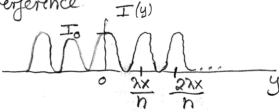
For a Young-type experiment with  $N$ -slits we have an  $N$ -beam interferometer based on division of wave front
