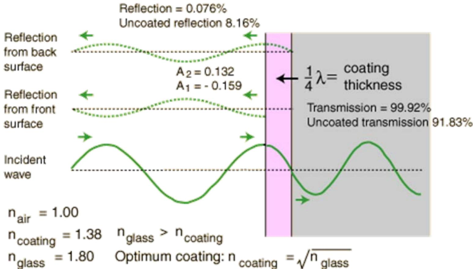
A limitation is that quarter-wave AR coating is designed for a given incident  $\lambda$  or  $\omega$  due to the condition
