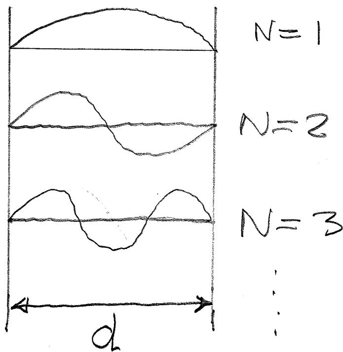
Longitudinal modes correspond to wavelength that fit into box of length  $d$ . Relevant concept for lasers, laser cavity length sets laser mode frequencies
