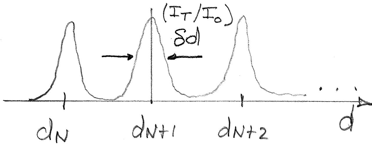
This can be used to measure  $\lambda$  for a source by scanning  $d$ .
