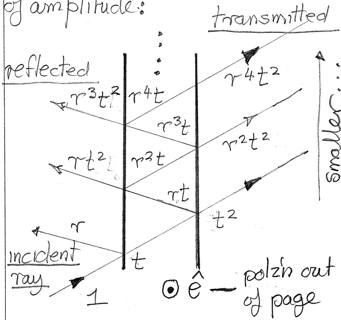
To get the total transmitted field due to an input field  $E_0$  (assume field is polarized out of the page) then we need to sum the partial waves
