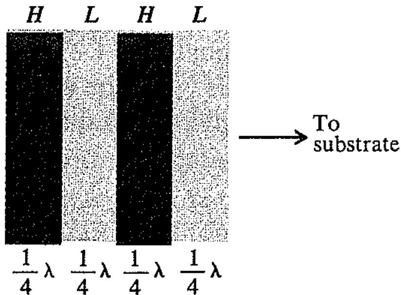
Multilayer stack for producing high reflectance. The stack consists of alternate quarter-wave layers of high and low index material. (Note:  $\lambda$  is the wavelength in the material.)
