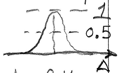
= 1 for  $\eta = 0$  (resonance). This falls to  $(1/2)$  for  $\eta = \pm 2/\sqrt{F}$ , so the FWHM of the fringes is.
