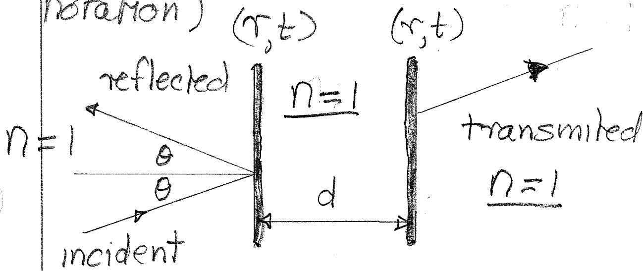
Incident harmonic wave of frequency  $\omega$  at angle  $\theta$  incident on pair of identical reflectors, or mirrors, of amplitude reflection coefficient  $r$  and transmission coefficient  $t$ .
