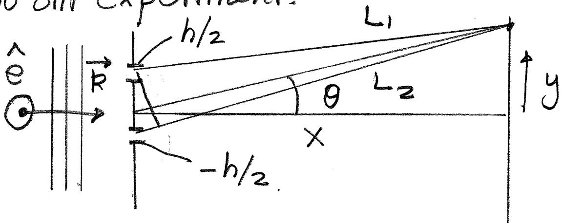
This is an example of a two-beam interferometer based on division of wavefront.
