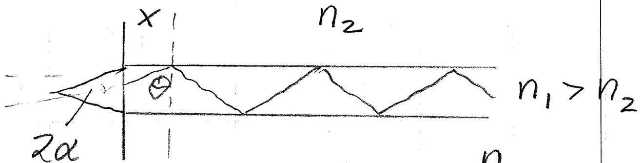
TIR provides confinement for range of input angles
