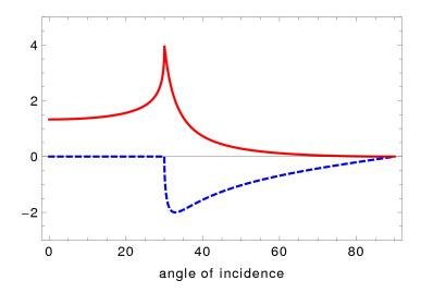
This picture shows real and imaginary part of a transmission coefficient.
