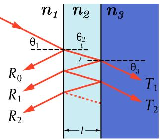
• Develop an intuitive picture of "what happens inside" of a multilayer. This will rely on the behaviors described by Fresnel equations, and in particular on phase changes experienced at reflections.
