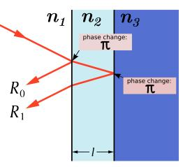
If, further, we adjust the thickness of the coating layer such that
