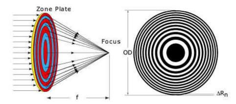
**Exercise:** In our derivation of the Fresnel zone radius, higher-order terms were neglected, resulting in an approximate expression for  $R_n$ . Derive the formula for the radius of the *n*-th zone of a zone-plate with a focal length f, this time without approximations, and show that it is:
