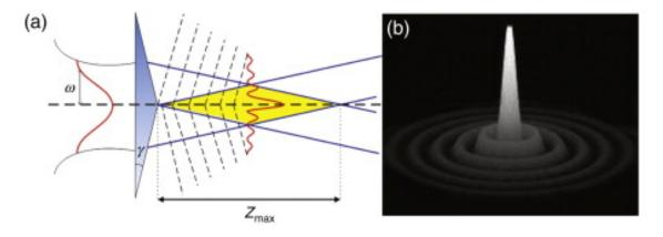
This is how they are created in practice. Nobody has infinitely wide plane waves, of course. Here the conical superposition is approximated behind a conical lens, axicon, but only within certain zone close to optical axis.
