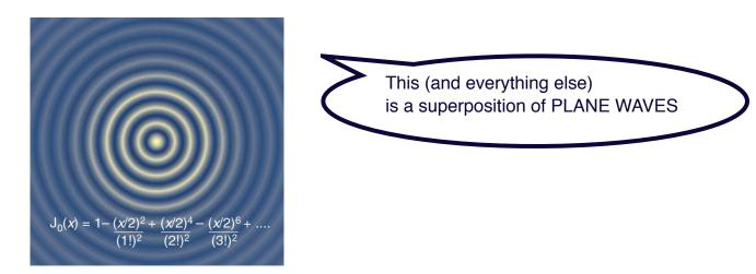
Transverse intensity cross-section of the Bessel beam. Each ring carries equal power.
